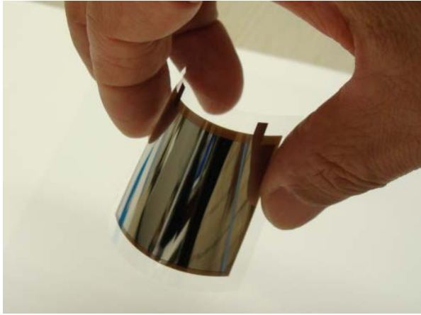
30- \mu\text{m} ultra-thin glass substrate lithium-ion secondary battery
