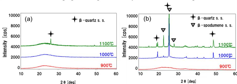
Figure 1. XRD pattern of heat treated (a) SnO<sub>2</sub> free and (b) SnO<sub>2</sub> added samples.
