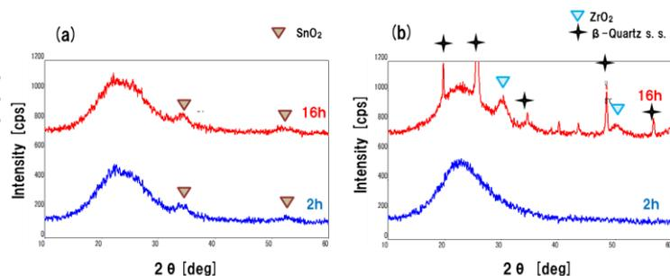
Figure 4. XRD pattern of (a) SnO<sub>2</sub> or (b) ZrO<sub>2</sub> added samples.
