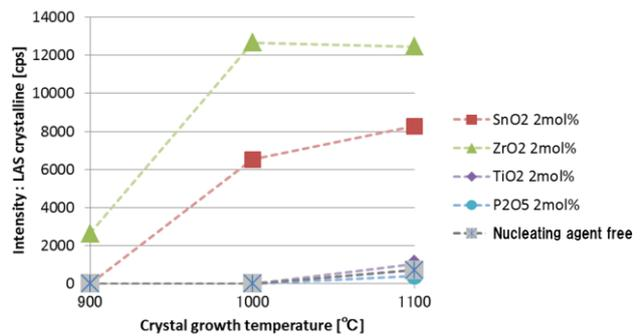
Figure 2. XRD intensity due to LAS crystalline changing nucleating agent.
