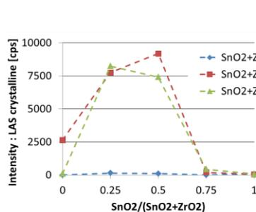
Figure 3. XRD intensity due to LAS crystalline of SnO<sub>2</sub> and ZrO<sub>2</sub> added samples.
