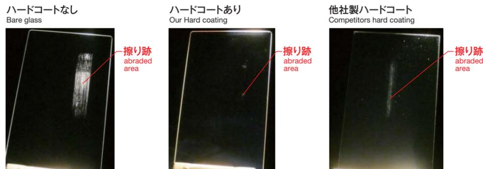
3M Garnet #150 sandpaper, load 2000gf, 16 cycles/min, stroke 40mm, contact 10mmx10mm, 100cycles.
