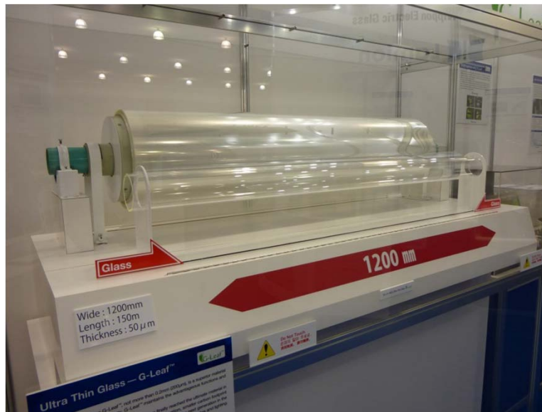
G-Leaf (Thickness 50 μm, Wide 1200mm, Length 150m)
