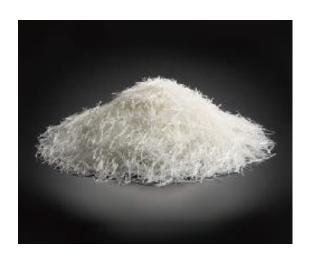
H-103 chopped strands are a loosely bound strand type so as to meet the dispersion requirements of plastering / rendering with cement mortar. The fiber strands are broken down into individual filaments during mixing, and works to prevent crack propagation even when used at a low dosage.
