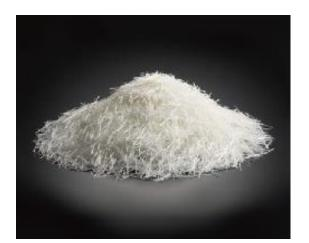
H-950X chopped strands is a high integrity type of medium tex strands. It has excellent strand integrity to meet requirements of a conventional premix GRC. The medium tex strands can achieve a balanced performance with good moldability and reinforcing effect at high dosage.
