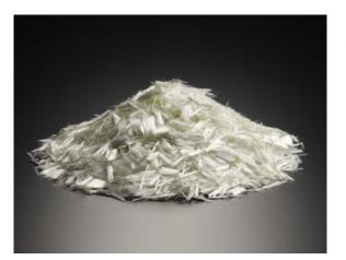
PS-750 chopped strands is water dispersible type used for water rich cementitious slurry / cement mortar. It contains some moisture and immediately disperses well in water / cementitious slurry and works as crack control at low dosage.Its filament diameter is 18 micron which is higher than S-750 chopped strands.
