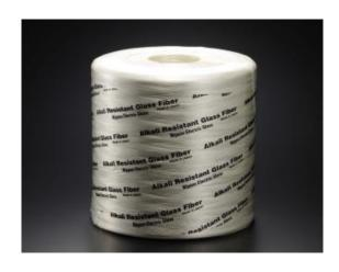
H-103 roving is the standard multi-end assembled roving, developed for the spray-up process. Its unique semi-integrated sizing system achieves good impregnation of the chopped fibers into cement mortar. Its softness and supple fiber strands are suitable for intricately shaped product designs.
