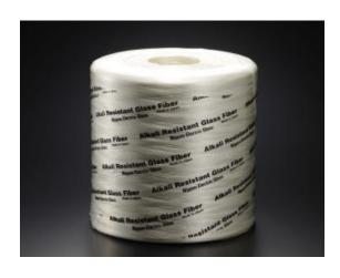
H-960 roving is multi-end assembled roving developed for excellent performance for GRC. It is especially for use with intricately shaped products in a spray-up process. The unique sizing system promotes conformity to the mold surface without bridging and creates a smooth surface.
