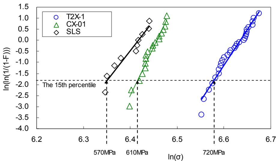
Figure 5. Weibull plot of T2X-1, CX-01 and SLS.  $\sigma$ [MPa] is fracture strength. F is failure probability calculated by Mean ranks.
