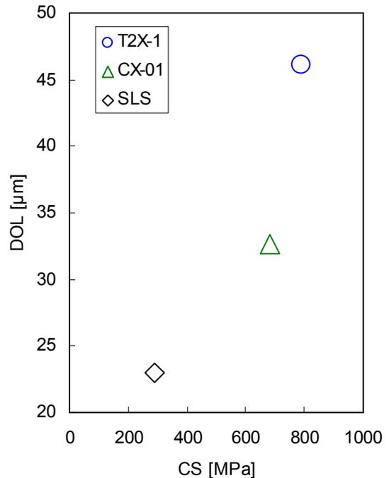
Figure 4. DOL and CS of T2X-1, CX-01 and SLS, ion exchanged in KNO<sub>3</sub> molten salt (Na<sup>+</sup> ion concentration: 6000ppm) at 430°C for 4 hours.
