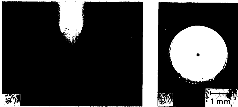
Fig.3 Outlook of cerammed preform redrawing a) : Neck down area b) : Cross-section of the micro-capillary
