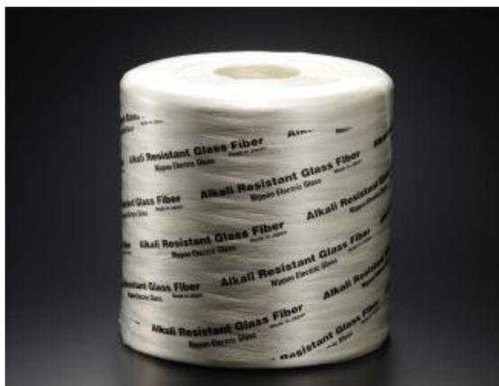
H-530X roving is multi-end assembled roving specially developed for premix GRC to save transportation cost. It shows excellent chopping performance. Due to the high integrity of the strands it performs very well in a premix process. It can also be used for spray-up process.
