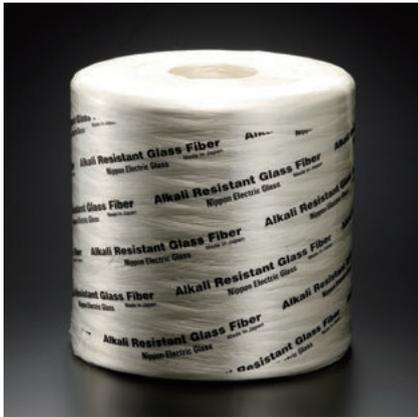
AR2500H-200 roving is made of glass fibre, which contains more than 16% of  $ZrO_2$ . AR2500H-200 is made by gathering 200 filaments into a strand, then winding 32 strands to form a cylindrical package.
