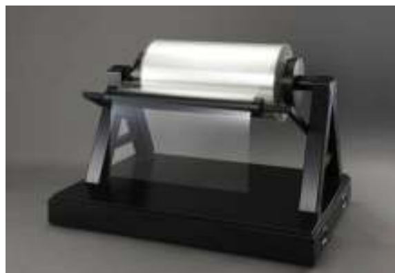
Figure 1 A photo of ultra thin glass roll.
