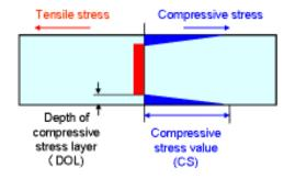
Figure 2. Schematic illustration of compressive stress laver.
