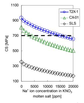
**Figure 7.** CS of T2X-1, CX-01 and SLS versus Na<sup>+</sup> ion concentration in KNO<sub>3</sub> molten salt.
