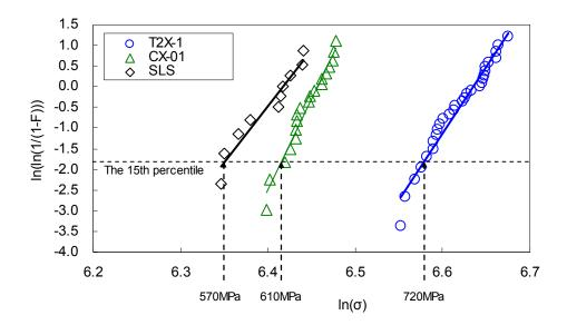
Figure 5. Weibull plot of T2X-1, CX-01 and SLS. o[MPa] is fracture strength. F is failure probability calculated by Mean ranks.
