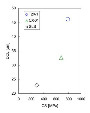
**Figure 4.** DOL and CS of T2X-1, CX-01 and SLS, ion exchanged in KNO<sub>3</sub> molten salt (Na<sup>+</sup> ion concentration: 6000ppm) at 430°C for 4 hours.
