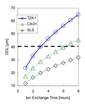
**Figure 6.** DOL of T2X-1, CX-01 and SLS versus ion exchange time.
