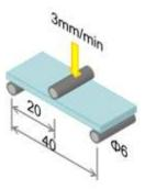
Figure 3. Schematic diagram of three-point-bending test.
