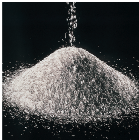
E-fiber for engineering plastics: chopped strands Glass fiber is chopped into tiny pieces, which are molded into automotive parts by injection molding after being processed into a compound mixed with plastic.
