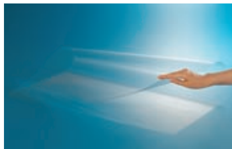
Ultra-thin sheet glass folded in the middle
