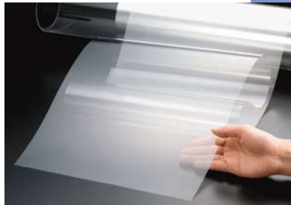
Highly flexible ultra-thin glass sheet
