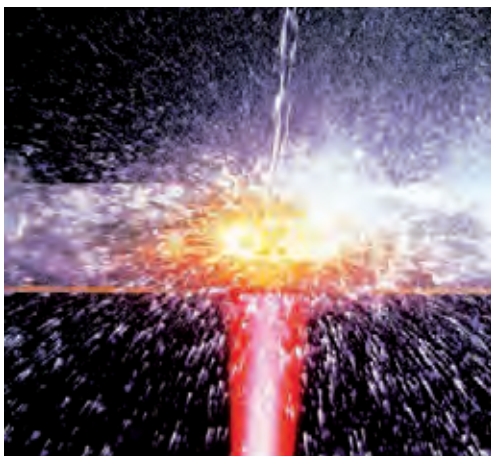
Thermal shock resistance test: glass does not break even when heated to 800°C and splashed with water.
