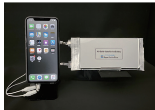
Test charging of a smartphone using the sodium-ion battery
