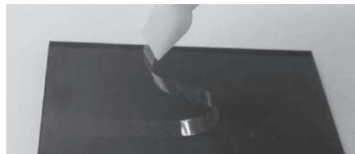
A fabricated all-glass-based microchip
