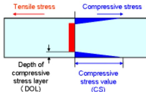
Figure 2. Schematic illustration of compressive stress layer.
