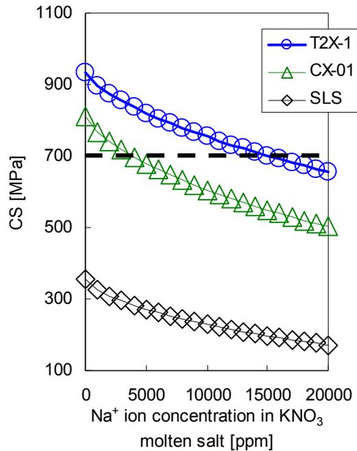
**Figure 7.** CS of T2X-1, CX-01 and SLS versus Na<sup>+</sup> ion concentration in KNO<sub>3</sub> molten salt.
