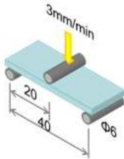
Figure 3. Schematic diagram of three-point-bending test.
