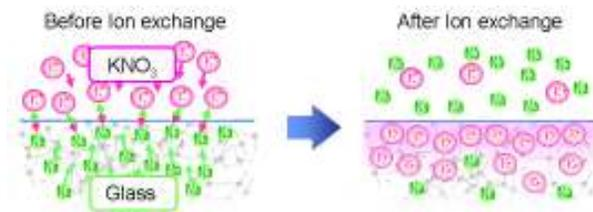
Figure 1. Schematic illustration of ion-exchange.
