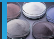
Granulated glass for metal packages
