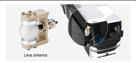
A lens antenna made with special glass, developed by Nippon Electric Glass Co., Ltd. (Head Office: Otsu, Shiga, Japan), has been used in a self-driving bus convoy experiment conducted in Shiga Prefecture, Japan.
