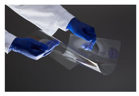
The special glass Dinorex UTG<sup>™</sup> (ultra-thin glass for chemical strengthening) used in the Alpair 5G. Although it is glass, it is only 0.025 mm (25 µm) thick at its thinnest and can be bent to a diameter of 3 mm (radius of 1.5 mm) or less.
