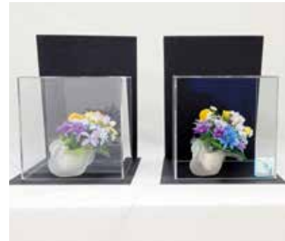
普通のガラス(左)、反射防止膜付きLamion™(右) Bare glass (Left), Anti-Reflection coated Lamion™ (Right)
