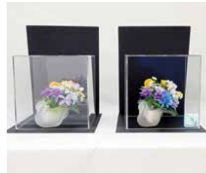
Bare glass (Left), Anti-Reflection coated Lamion™ (Right)
