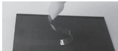
A fabricated all-glass-based microchip
