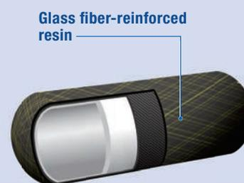
On-board hydrogen tank protected by a surface layer of glass fiber-reinforced resin
