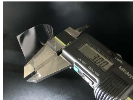
Bend with a diameter of 3 mm (R1.5) made possible
